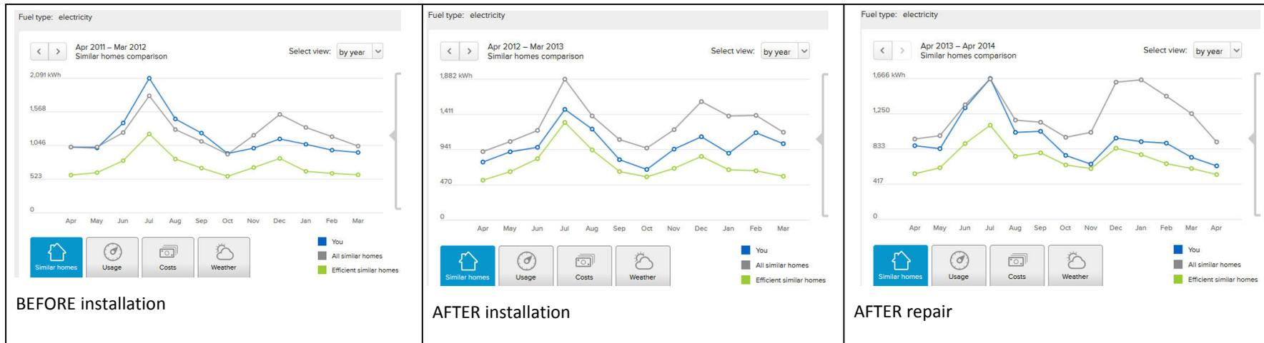
The first year April 2011 – March 2012 shows the consumption pattern before the standard electric water heater was replaced. The home's electric usage follows the pack of similar houses with slightly better performance. The electric water heater has an EF of .91, typical of many homes.
